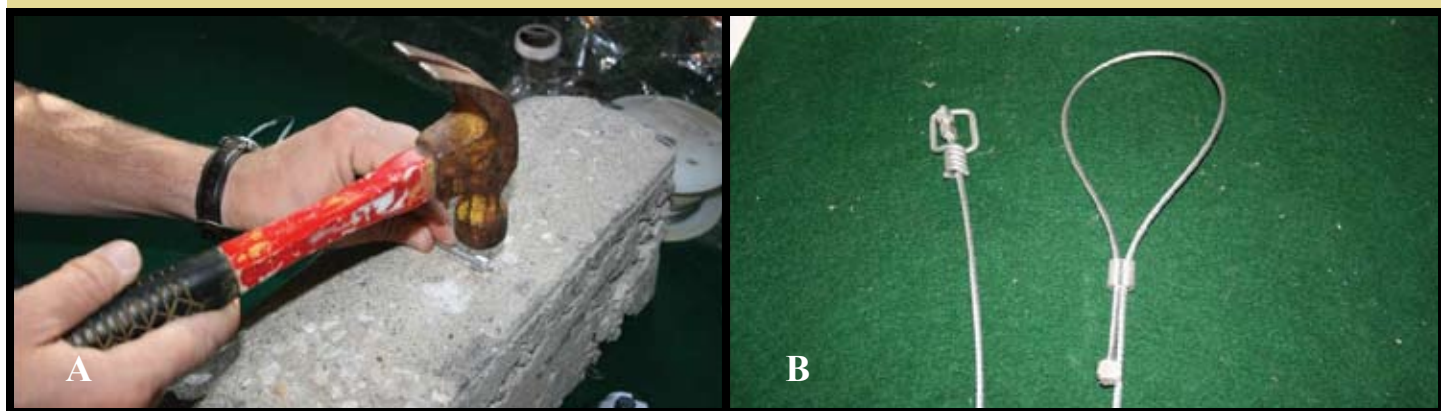
Figure 8. Attach a ferrule to the end of the cable (A). The snare can be designed with a swivel end (B, left) or an adjustable end (B, right).
