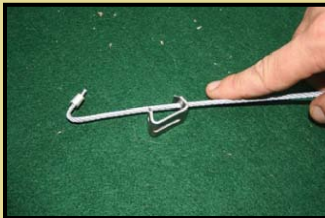
Figure 4. Reverse bend above single ferrule to secure snare lock.
