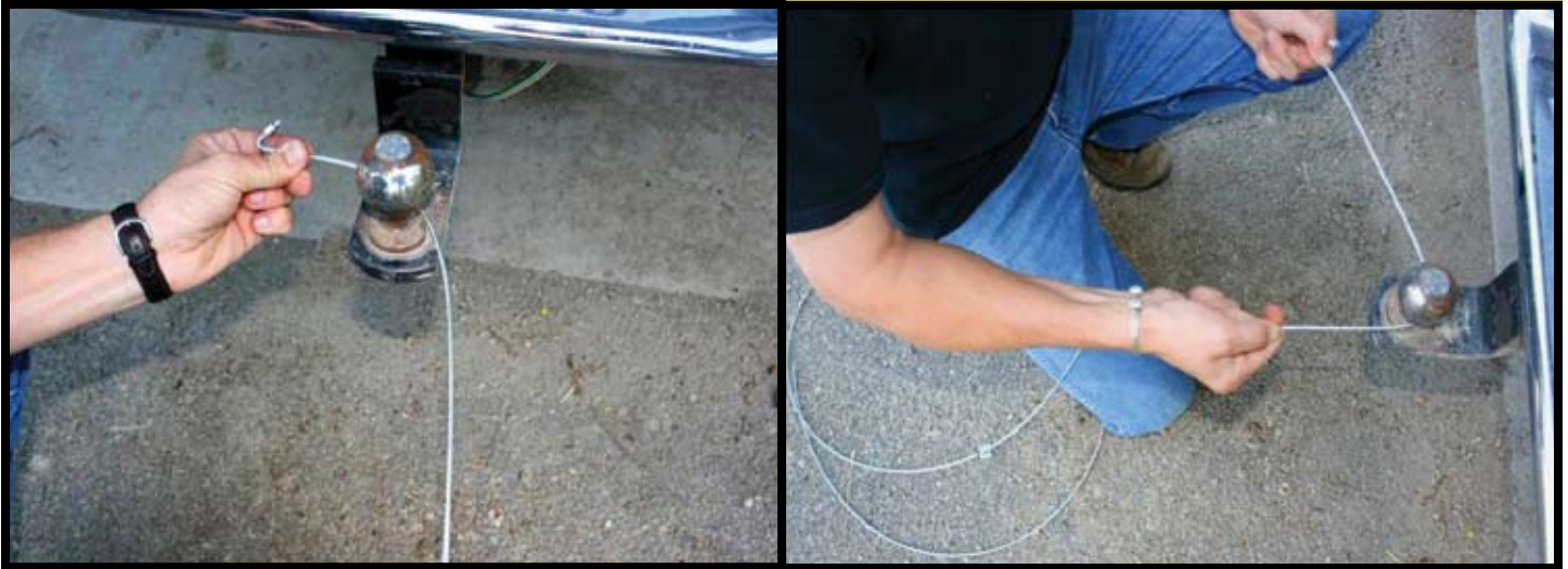
Figure 5. Load the snare by applying pressure as the cable is moved back and forth.
