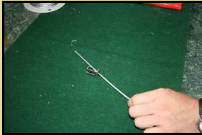
Figure 2. Begin by running the cable through the snare lock.
